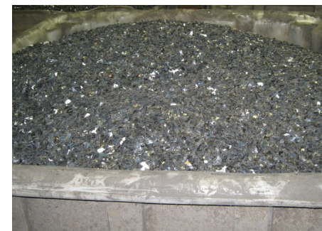
Film is shredded into flake and the silver is separated from its plastic backing.
